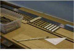
Once my sleepers are dry and ready to lay, I set out a datum line on the section of the layout using the edge of a steel straight edge – of course this is only applicable for straight track. I like to use a centre line for track laying rather than relying on the edge of the sleepers as a guide because some of them are longer than others. I paint the back of the first sleeper with a
