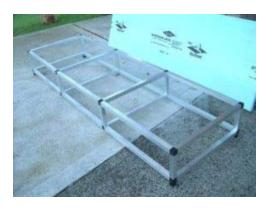
On top of the frame I have added a track baseboard comprising sheets of 30mm thick extruded foam which have strips of 6mm thick MDF glued to their underside to provide a screw fix to the aluminium frame, making the whole thing able to be dismantled easily.
