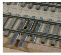
This photo shows the thin end of the switch rails and the spreader bars in place. I had to come back and readjust these which is the reason you can see bare solder; once painted all this will blend in. The spreader bars extend under the rail to ensure there is no chance of the switch rails lifting or springing out of position.
