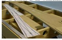
This photo shows a little more clearly the arrangement of the 3mm MDF "insert" that I'll build the point on and eventually pin into place after the point has been completed. Those wooden sleepers have been glued into place and I'll fill in the gap with more a little later.
