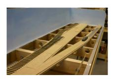
In this photo (which is a different point to some of the earlier photos), you can see where I've installed the 3mm MDF insert with the point in place and have laid some more sleepers up to the edges of the point. I'll lay rail on the plain track starting from the point and working outwards. The sleepers are laid using PVA.
