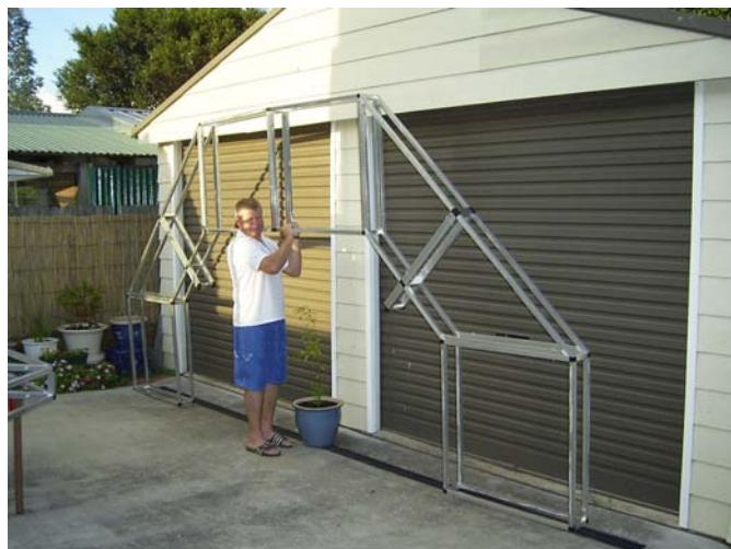
Left :Detail of corner module showing bracing required for backdrop and lighting rig
