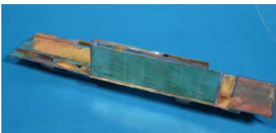
This footplate was built to demonstrate the quality and ease of construction of the proposed 20 class
