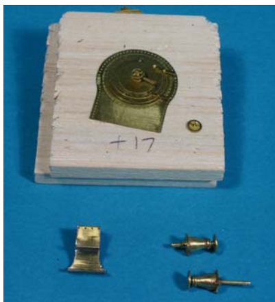
Smoke box door, steps and buffers for the 20 class.
