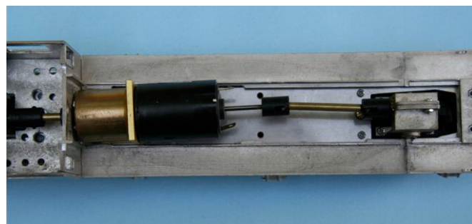
Photo 1. Relocated motor and skewed drive shaft
