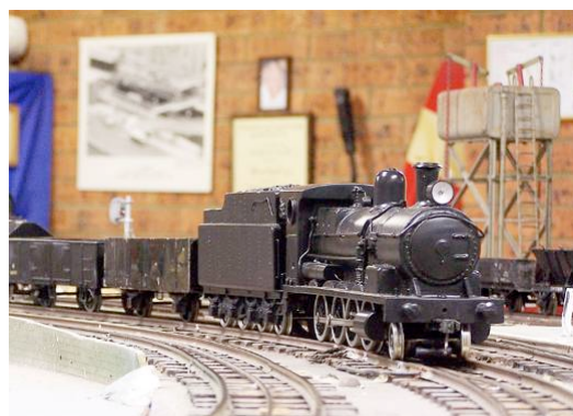
A Fox three-rail standard goods. The mechanism was made especially for the owner, using wheels and bearing block by C. Shepherd, G. Taylor collection.
