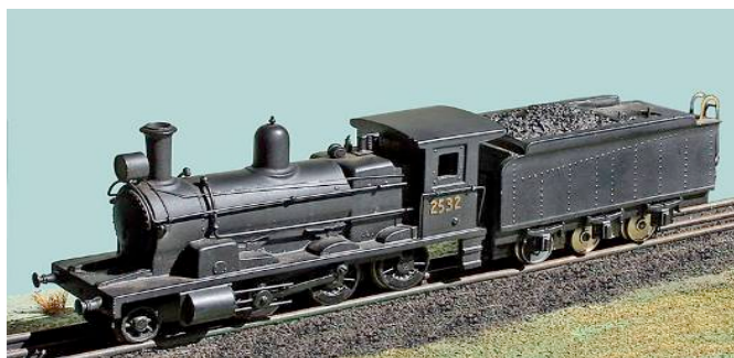
A Fox 25 class fitted with an Atlas 6-wheel tender drive, G. Taylor collection.
