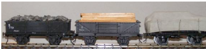
The ubiquitous 4-wheel S open wagon carried a diverse range of goods from sawn timber to crushed rock. Some goods needed to be protected from the environment by draping a tarpaulin over them.
