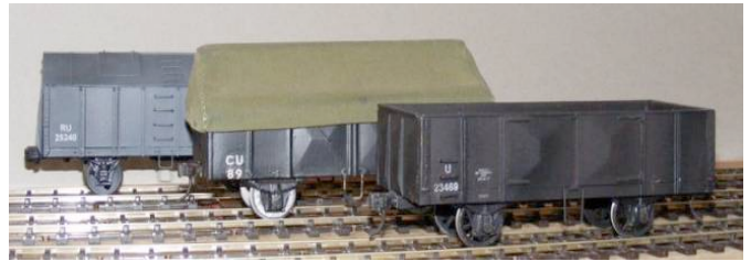
Variations on a theme. Modification of the basic 4-wheel U open wagon. The basic 4-wheel U open wagon; the CU 4-wheel open wagon was permanently fitted with a ridge pole and tarpaulin; and the enclosed RU 4-wheel wheat hopper wagon.
