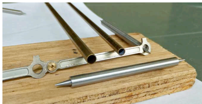
Above: The 3/16" OD and 5/32" OD size tubing, the coupling rods and a 3/16" alignment axle with tapered ends for using with the normal 3/16" axle size and tapered various sized coupling rod bearings, the size of which in this instance is way too small for the coupling rod bearing holes that are 5/32" in diameter on this particular model.
