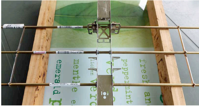
Above: Plan view of chassis, tubular axes with coupling rods fitted for aligning the axles.
