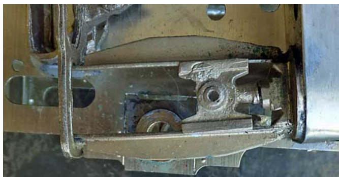
Above: Slide bar effectively prevents insert of front driving axle.
