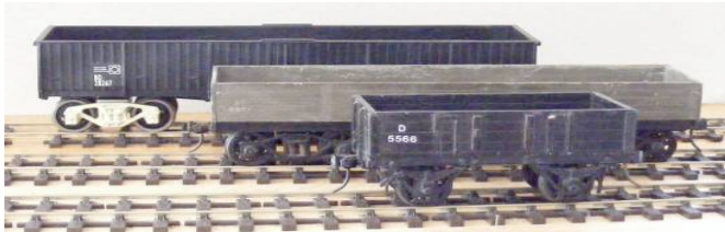
Evolution from the small 4-wheel D open wagon, into the larger bogie BD open wagon with timber sides, into the larger bogie BD open wagon with vertically ribbed steel sides.
