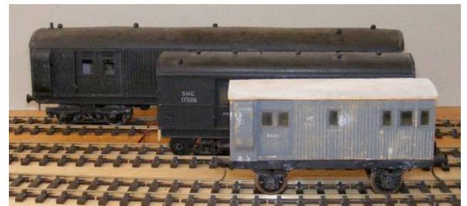
Variations on the need to provide passenger accommodation for a few passengers along lines where there were too few passengers to justify running a separate passenger train. The small 4-wheel HG, the larger bogie SHG, and the larger bogie LHG guards vans are just a few of the diversity.
