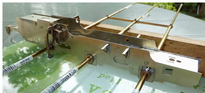
Right: Side view of chassis and tubular axles in place.
