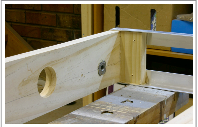
2. The inside corner of the Queens Wharf module. The length of 2X1 acts as re-reinforcement for the corner and gives more surface area for the glue and screws to grip in this vital area. One of the T-nuts is visible close to
