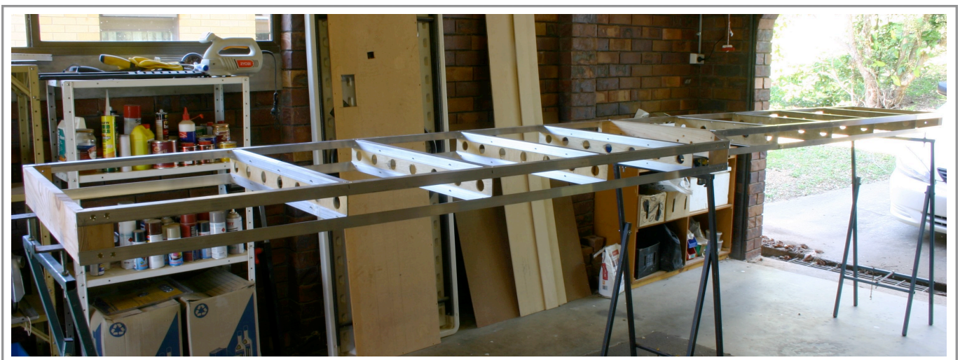
9. This photo shows two of the modules connected up and sitting on their stands. The overall saving in weight over the Queens Wharf modules is approximately 35%.
