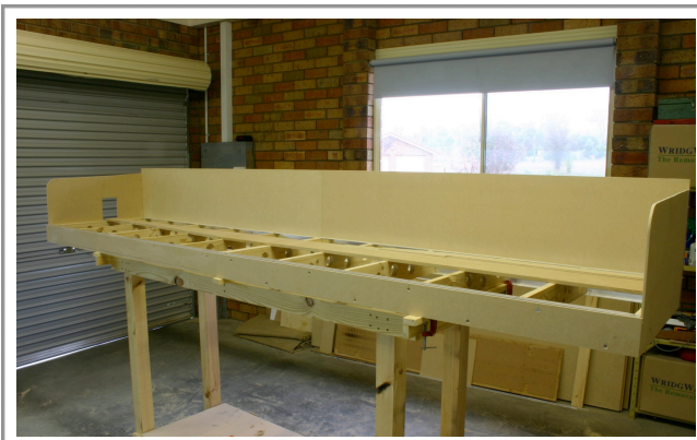
3. This is the layout in full and wrapped in a skin of 6mm MDF. The front fascia is made up of two pieces of MDF, one slightly narrower than the other, to provide a slot for the backdrop on the other module to drop into.
