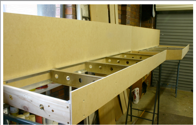
10. The 6mm MDF is secured with small bolts and nuts through holes drilled in the aluminium angle.
