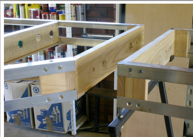
8. Joining the modules is precise with the use of pattern makers dowels. The ones pictured are from Station Road Baseboards in the UK.
