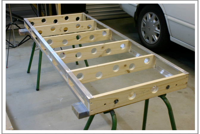
1. This is the base of one of the Queens Wharf modules. The modules are 1.5mX600mm in size. When the two modules are connected they form an extremely rigid grid which is more than adequate to hold trains off the ground.
