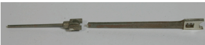
photo 10. piston rod and connecting rod assembly
