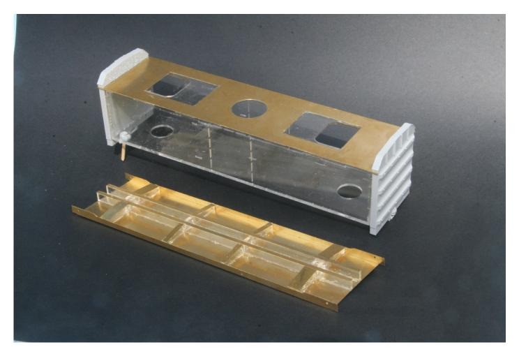
without any clean up or filing being required. The "box" provides a perfectly straight and square base structure for the subsequent attachment of the etched sides and 3-D printed ends.
