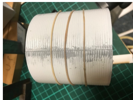
Photo 8 - filing the aligned corrugations.
