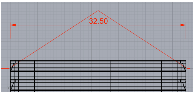
Figure 10.0 - The roof profile is extruded to form a solid model in the same way the plank was originally.
