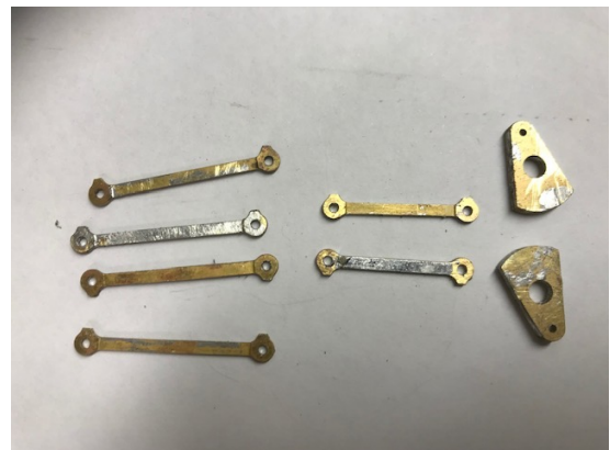
Photo 7 – rods and weights soldered.
