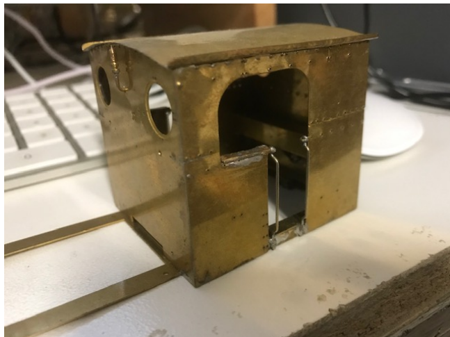
Photo 1 – cab with clean corners.
