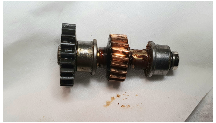
Truck drive shaft with worm gear and gear train gear. Build up of hardened grease shown.
