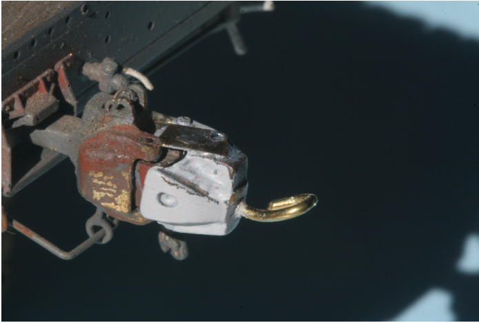
Photo 1. Adapter coupled to KF wagon
