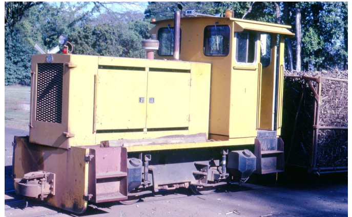
EM Baldwin 2ft gauge 4-wheel locomotive in yellow, Goondi (Innisfail) sugar mill No.1, 1 September 1980, D Mewes. Many EM Baldwin's had outside coupling rods. However this one opens up the potential for modelling outside framed locomotives as well, as happened to be the case with the two models herein.
