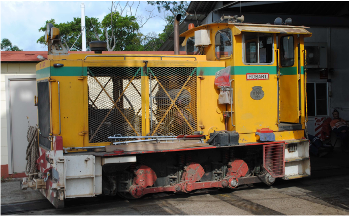
EM Baldwin 2ft gauge 6-wheel locomotive with outside connecting rods in yellow livery with a white roof, Macknade sugar mill, nd, J Browning. Note the storing of potentially useful items along the side foot board.
