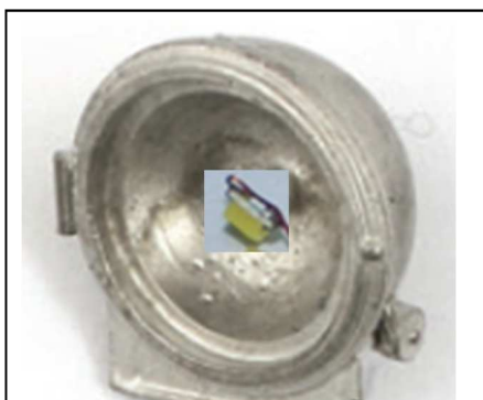
Prototype white LEDs can also be mounted directly into a headlight casting.
